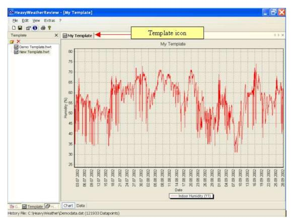
If you want to keep a permanent copy of this particular plot, just click button or select "Save as Graph" in pull down menu or press Ctrl-S to save it as a graph. The plot would become a graph plot immediately identified by its icon. You can also find its name listed in the graph file management window.
