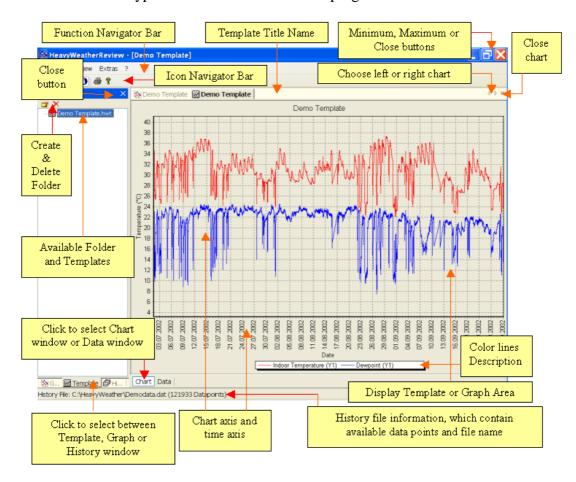
There are two main windows in above figure, the left one is the file management window which allows you to select and show the history, template or graph files. The right one is the chart/data windows which shows you the current plot or current data.
